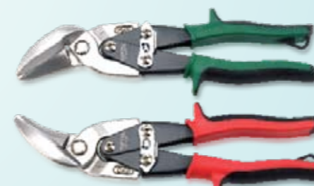
240mm Offset Tin Snips Drop forged chrome molybdenum alloy steel blades. Induction hardened cutting edges. Precision serrated cutting jaws
